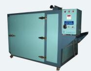
These are extensively used in food processing and other commercial Establishment for bulk drying of Grains, Corns, Food-stuffs and other products a Controlled temperature with high accuracy of performance. Added with forced air circulation this ensures maximum uniformity and quicker drying.
